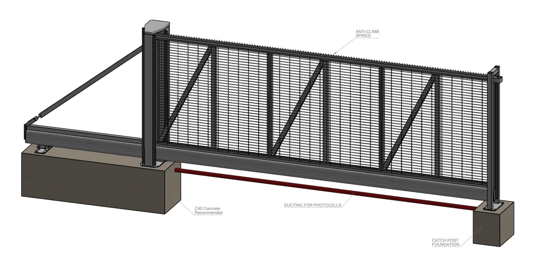
AUTO CANTILEVER SLIDING GATE 6000mm Opening x 2400mm High MESH - Left-Handed
